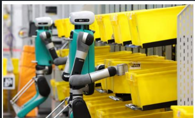
Digit, which can walk forwards, backwards and sideways and crouch, is 5ft 9in and carries up to 35lb. Photograph: Jason Redmond/AFP/Getty Images
